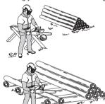
The log is lying on the ground. There is little risk of the chain jamming or the object splitting. However there is a risk that the chain will touch the ground when you finish the cut.
